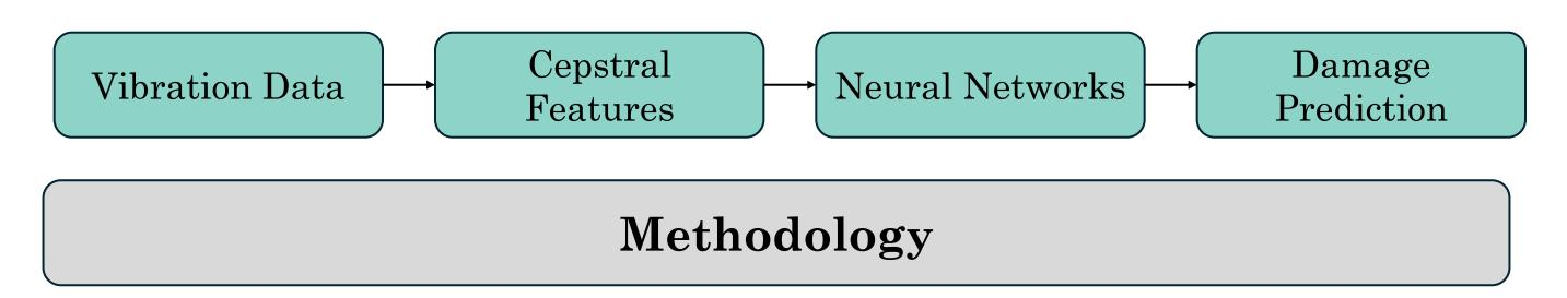
Feature Extraction: Cepstral Analysis captures frequency-domain characteristics of vibration signals, aiding in damage identification.
